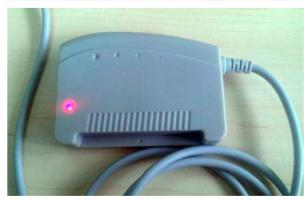
RT01A is a reliable and effective PC-LINK smart card reader/writer with a full speed USB interface for the communication between a computer and a smart card.
