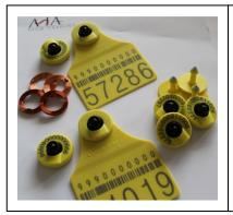
Asia Tech has developed along with its partner a full range of tags, fully compliant to the standard FDX-A, FDX-B, HDX covering any needs of this specific field.
